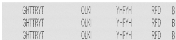
Figure 23. Example of reconstructed image from sensitive emission for a two-diode laser printer, 660dpi mode with the “Eco” option turned on. Measured frequency of sensitive emission: f_0 = 444 MHz, BW = 5 MHz. Image is inverted.
