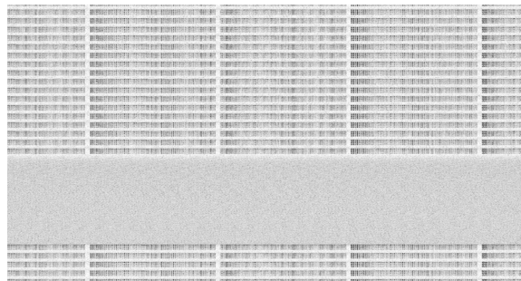
Figure 21. Fragments of reconstructed images from sensitive emissions of printer A: (a) 1200dpi mode without toner save, (b) 1200dpi mode with toner save, measured frequency of sensitive emission: f_0 = 525 MHz, BW = 5 MHz. Image is inverted.
