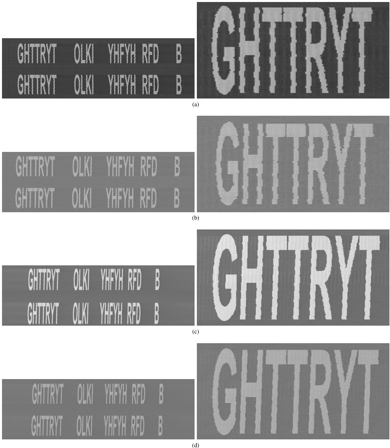
Figure 16. Examples of images recreated from useful signals (printer B ) for (a) 600 dpi without toner save, (b) 600 dpi with toner save, 1200 dpi without toner save, and (d) 1200 dpi with toner save.
