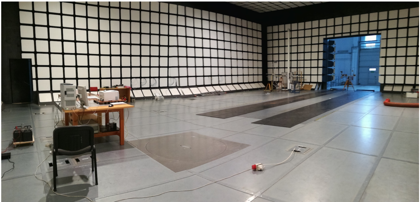
Figure 17. Anechoic chamber where the tests were carried out.
